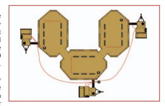
Digital smart systems allow personnel to connect multiple generators to run together as a single power grid and reduce fuel consumption. In the above field hospital, all generators are working together to power the facility as one grid.
