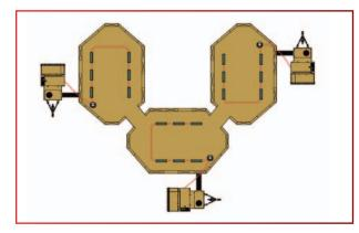
Generators running on "island mode." From a power perspective, the above field hospital is comprised of three separate facilities that each require its own generator and do not share any power lines. Even if one generator could satisfy the power needs of the entire hospital (example: at night when lights, medical equipment, etc. are turned off), all three must run at all times. This wastes fuel and creates unnecessary run-time hours.
