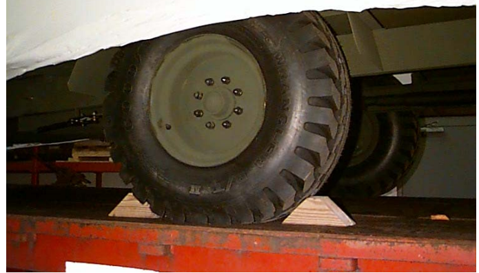
Figure 2-3 - Wheel Properly Chocked
