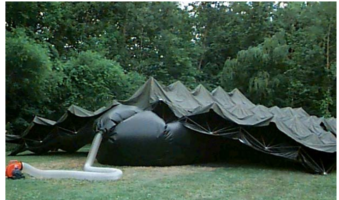
Figure 3-9 - Inflating Bladder Lifts Shelter
