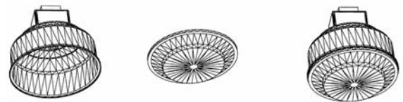
Figure 3-23 - Connect the Lens to the Reflector
