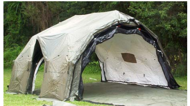
Figure 2-9 - Center Section in Erected Position
