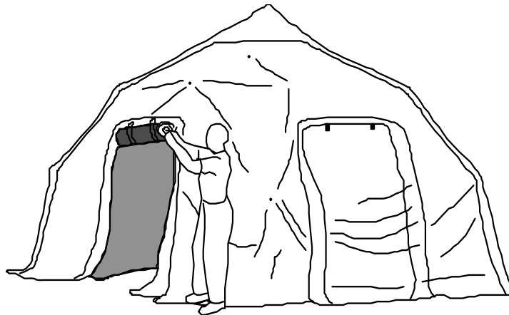
Figure 15. Tie Back Doorways
