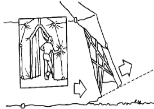
Figure 3-1 - Tie Back Doorways
