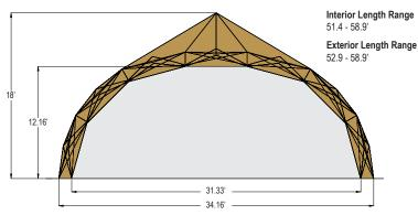
The DRASH design is **comprised of a frame with two pre-attached covers and a ground cover.** This means that setting up a DRASH<sup>®</sup> shelter does not require special tools or dealing with loose parts. Additionally, its easy-touse strut and hub configuration **allows it to be set up within minutes** of arriving at a location.
